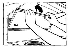
4. With both hands, carefully fit the glass light cover into the bottom metal support trim. Then rotate the top of the light cover until it touches the contact stops. Replace the top support trim and 3 screws. Plug in appliance or reconnect at the main power supply.
