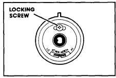
Loosen the locking screw inside the control knob. Note the position of the notches.
