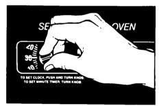
Without pushing it in, turn the Minute Timer Knob until the time in the window passes the setting you want.
