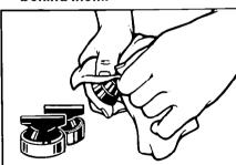
Wash control knobs and surface unit collars in warm soapy water. Rinse well and dry. Do not soak.
